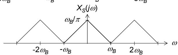
$T_S = 2\pi/\omega_B$ ,  $\omega_S = \omega_B$ :
