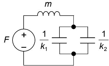
**P19.1.4** The equivalent electric circuit is a series combination of  $L$ ,  $C_1$ , and  $C_2$ .
