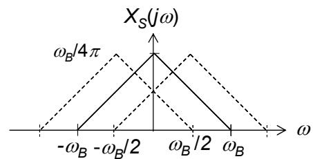
**P17.4.4** The sampling rate must be equal to twice the 1 rad/s bandwidth of the signal, i.e., 2 rad/s.
