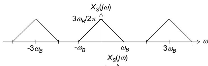
$T_S = \pi/\omega_B$ , or  $\omega_S = 2\omega_B$ :
