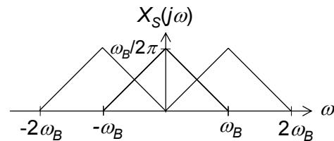
**P17.4.3** The frequencies that are adequately sampled are those in the range 0 to  $\omega_S/2 = \omega_B/4$ . The frequencies are folded back around this frequency.
